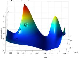
Figure 7. The objective function for the simplified model, as a function of two variables: log(generation rate) on the x-axis and log(permeability) on the y-axis. Between 17.0 and 15.5 it shows some point-like discontinuities that probably are caused by numerical instabilities in the forward model
