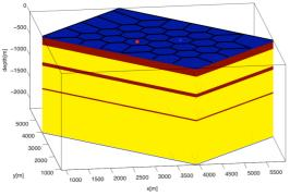
Figure 4. 3D view of the model. Colors correspond to different material properties The blue and red points at the top layer represent the location of hot spring (water sink) and an observation well respectively.
