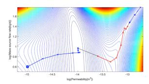
Figure 9: AKMC minimization path from initial guess represented as a blue square. It converges to the global minimum (path in blue), given an initial displacement (black dotted line) it climbs up to converge to the saddle point (path in red), given a displacement from saddle point (black dotted line) it converges also to the local minimum.
