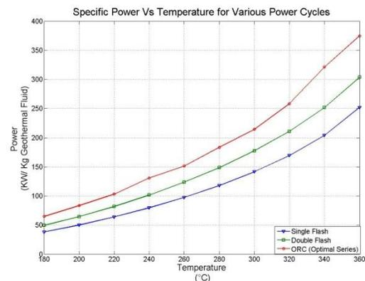
Figure 7: Specific power vs. temperature for the single-flash, double-flash and optimal organic Rankine series.
