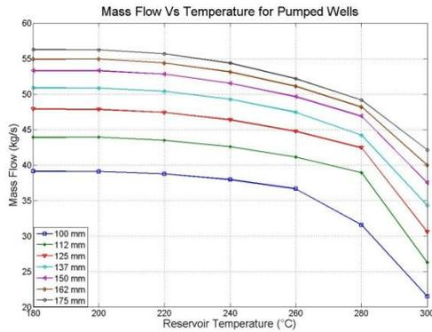
Figure 9: Mass flow vs. reservoir temperature for the pumped wells with various production tubing diameters.
