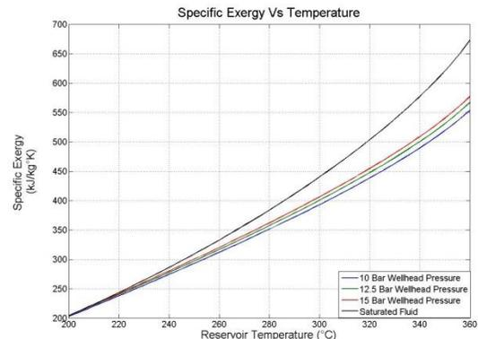
Figure 1: Calculated available specific exergy for a geothermal fluid at saturation pressure as well as 10, 12.5 and 15 bar wellhead pressure.
