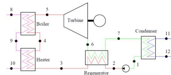
Figure 4: Process diagram for an ORC power plant with recuperator. (Pálsson, 2009)
