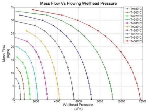
Figure 8: Mass flow vs. flowing wellhead pressure for various reservoir temperatures.
