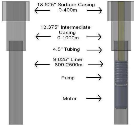
Figure 6: The two wellbore configurations used in the study.
