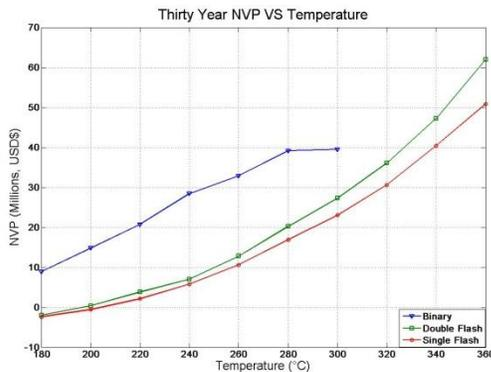
Figure 12: Net present value vs. reservoir temperature for various power generation techniques.
