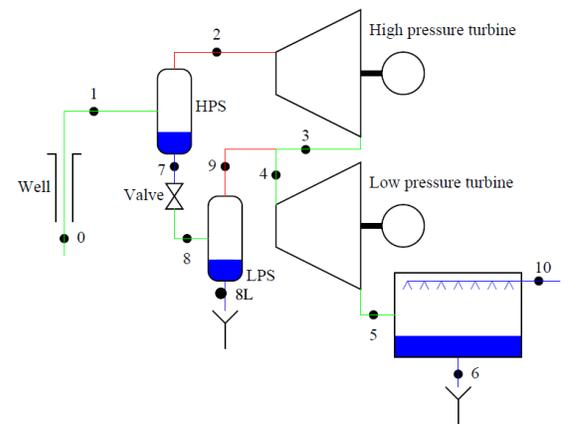
Figure 3: Process diagram for a double-flash power plant. (Pálsson, 2009)
