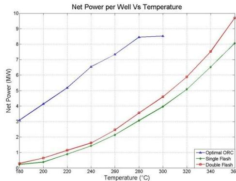
Figure 10: Net power per wellbore vs. reservoir temperature for various power generation techniques.
