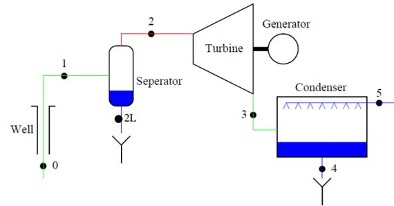
Figure 2: Process diagram for a single-flash power plant with condenser. (Pálsson, 2009)
