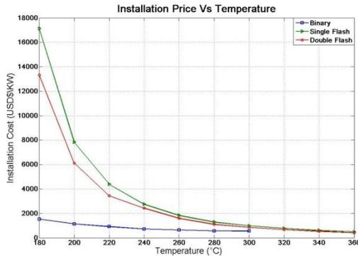
Figure 11: Installation cost vs. reservoir temperature for various power generation techniques.
