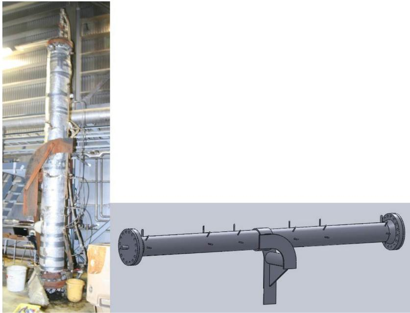
Fig. 6. A photo showing the experimental setup and a 3D drawing showing the pipe on the steel bracket.
