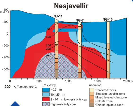
A simplified resistivity cross-section from Nesjavellir geothermal field, SW-Iceland (from Árnason et al., 1987). The zones of dominant alteration minerals are shown and temperature in nearby wells. The resistivity structure correlates fairly well with the alteration mineralogy.
