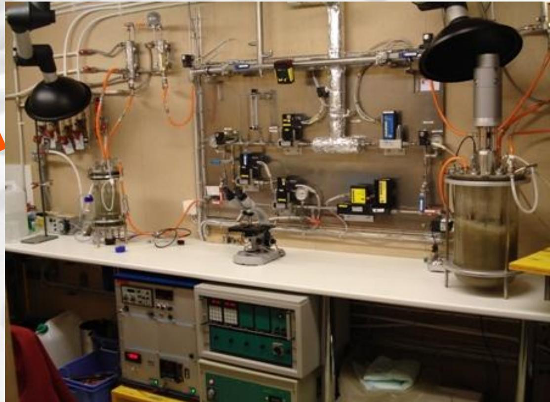
Cultivation of microbes on gasses directly from a geothermal powerplant
