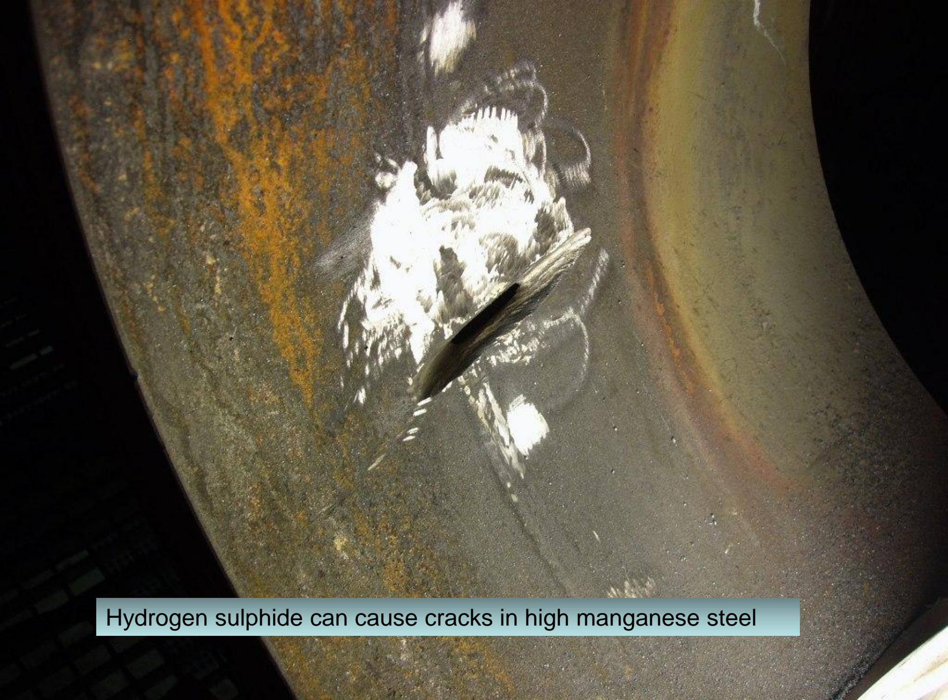
Hydrogen sulphide can cause cracks in high manganese steel
