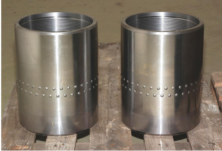
Prototypes of Flexible Couplings for 9 5/8" casings
