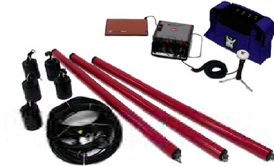
Figure 6.4. Phoenix V5-2000 MT system. From left to right; five non-polarizing electrodes, 3 induction coil cables, 3 MTC-50 induction coils, battery, MTU-5 recording unit, GPS antenna, and case for the unit. The picture is taken from Phoenix Geophysics web site.
