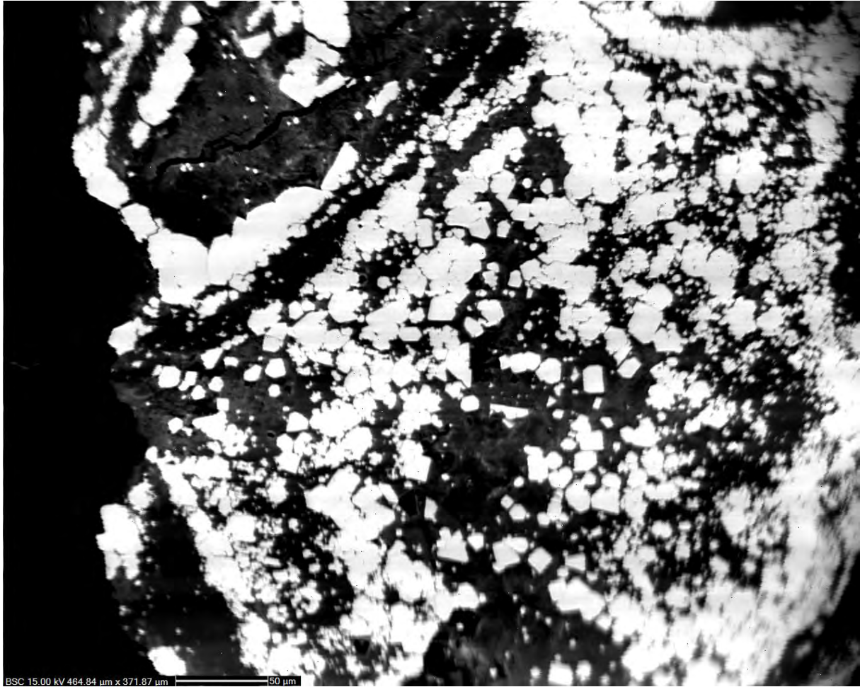
Figure 6. Sample from well HE-42, 558 m depth. SEM microphotograph, 15 kV. The base of the figure is 500 micron. Initial pyrite formation within a pseudomorph of pyroxene. Clustering and growth of crystals along edges of the pseudomorph. This is taken as an indication of fluid transfer of sulfide into the iron source material.
