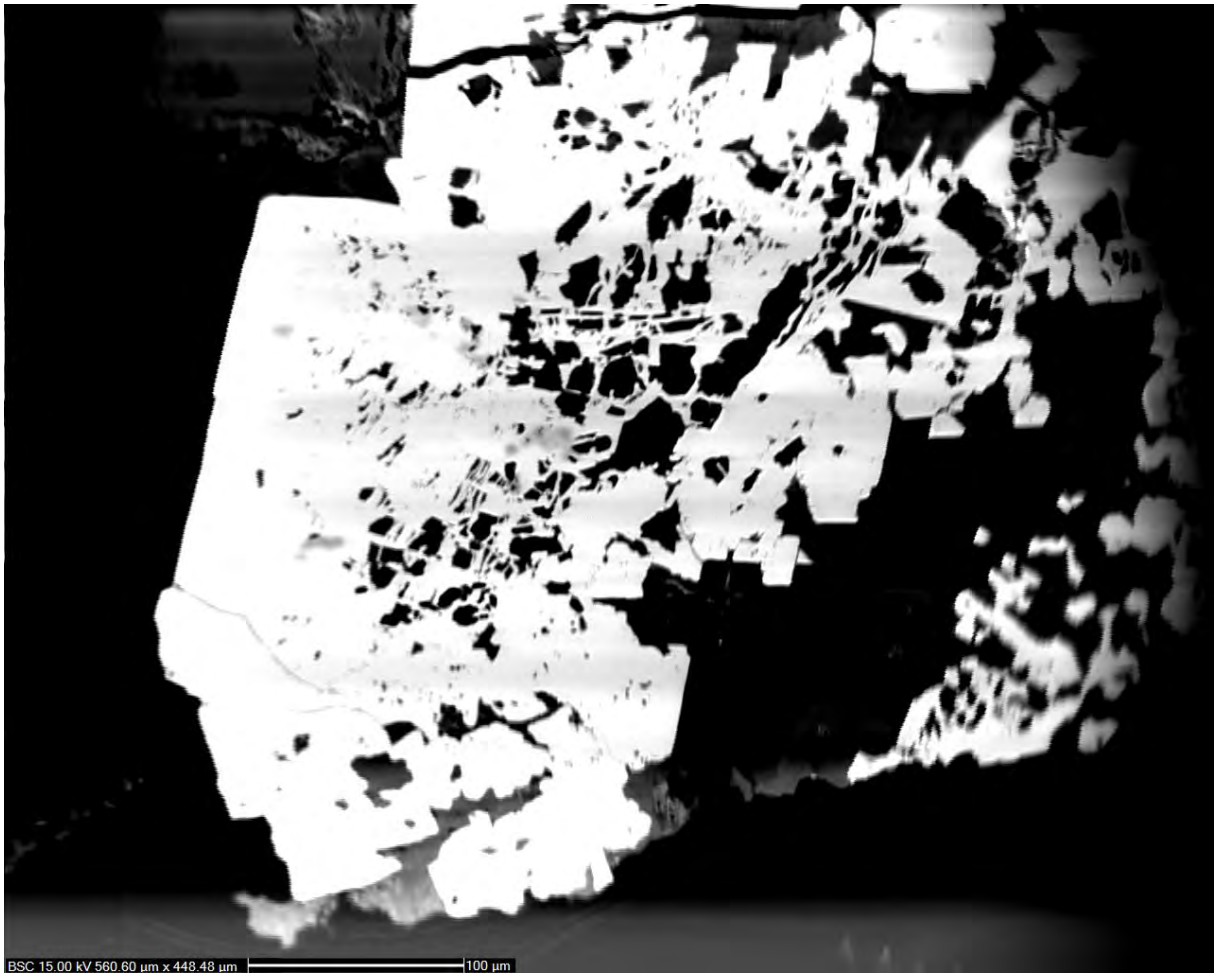
Figure 7. Sample from well HE-42, 512 m depth. SEM microphotograph, 15 kV. The base of the figure is 500 micron. Pyrite cluster evolving into a large euhedral crystal. The most common occurrence of euhedral forms is within cavities and clay-filled domains in the host rock.
