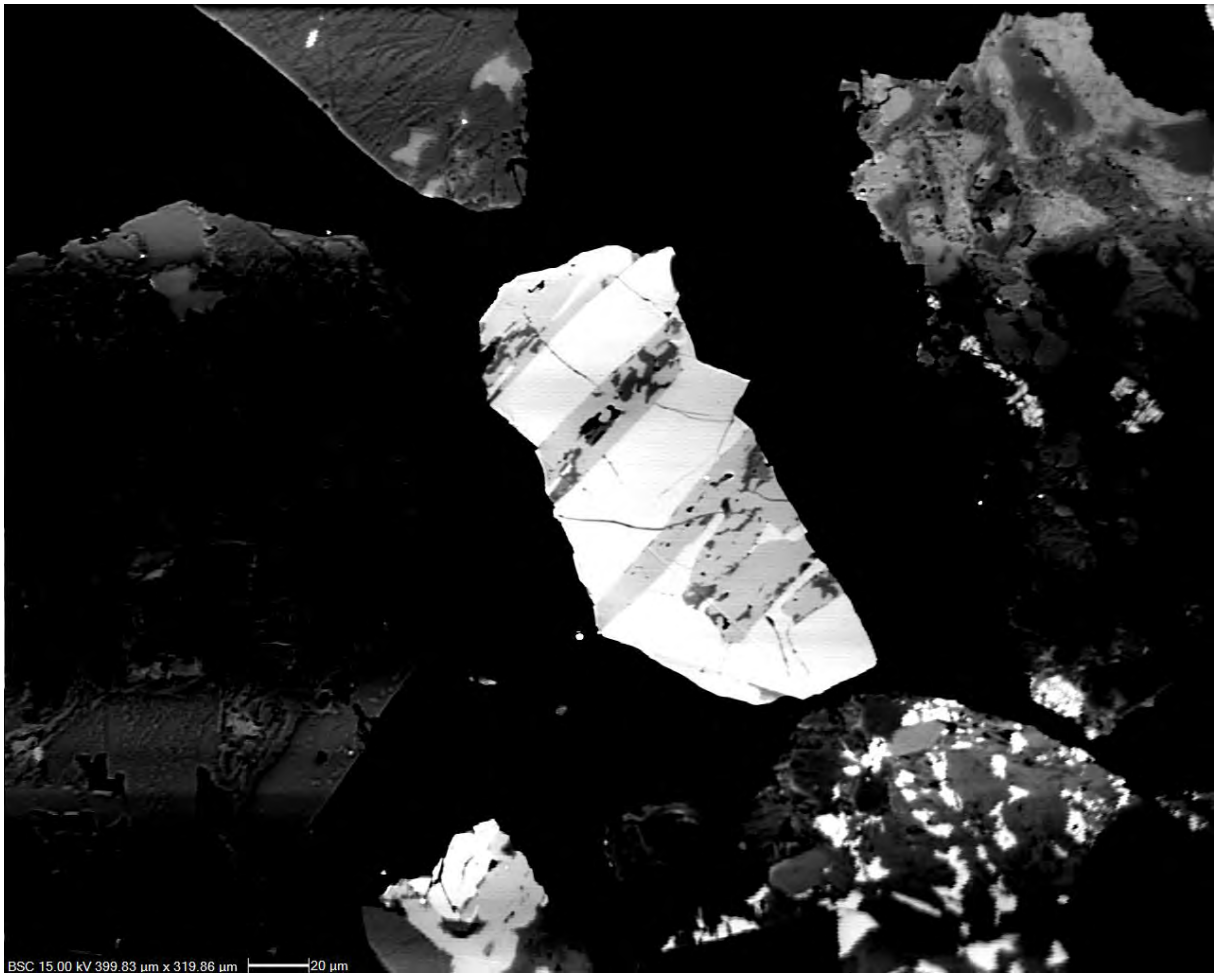
Figure 10. Sample from well HE-42, 1246 m depth. SEM microphotograph, 15 kV. The base of the figure is 400 micron. Ilmenite lamellae (dark) in titanomagnetite showing early dissolution pits. Most samples show clear signs of ilmenite dissolution although virtually fresh titanomagnetite with ilmenite exsolution may be found in cuttings from dykes and intrusions. This may reflect restricted permeability that isolates rock-domains from interaction with the geothermal fluid.
