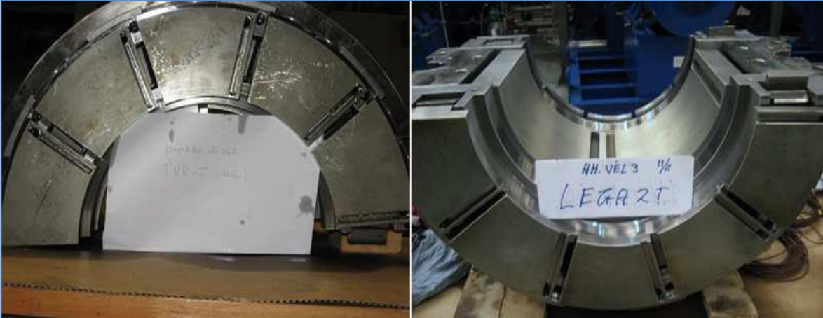
Figure 4.20 Left, pressure bearing from turbine 1 at Hellisheiði power plant. Right, one half of a main bearing for turbine 3 at Hellisheiði power plant [41].
