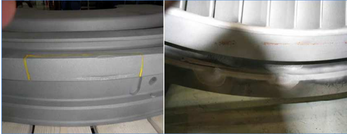
Figure 4.11 Both pictures are from turbine 2 at Hellisheiði power plant. Left, wear on the side and on the bottom of the third stage diaphragm. Right, wear at the side of the fourth stage diaphragm [41].
