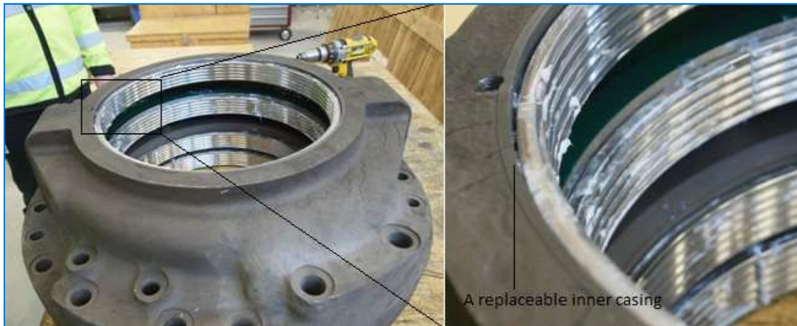
Figure 4.29 Left, repaired casing with new labyrinth packing made by Vélvík and a new replaceable inner casing made by Framtak. Right, an enlarged view of the new inner casing.
