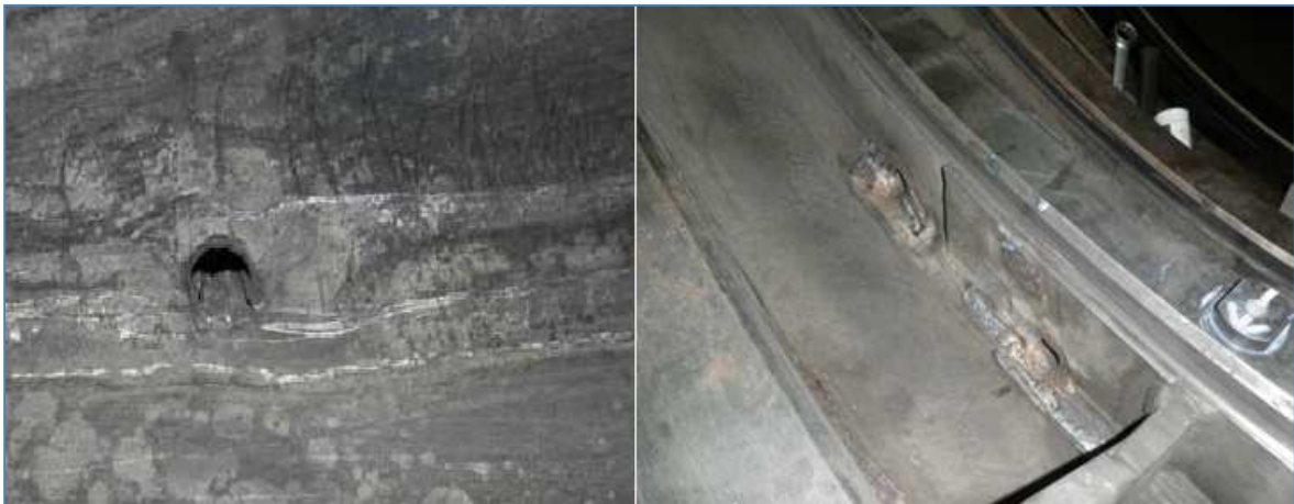
Figure 4.19 Left, wear of a drain hole at the third stage in turbine 2 at Hellisheiði power plant. Right, wear of drain holes in turbine 3 at Hellisheiði power plant [41].
