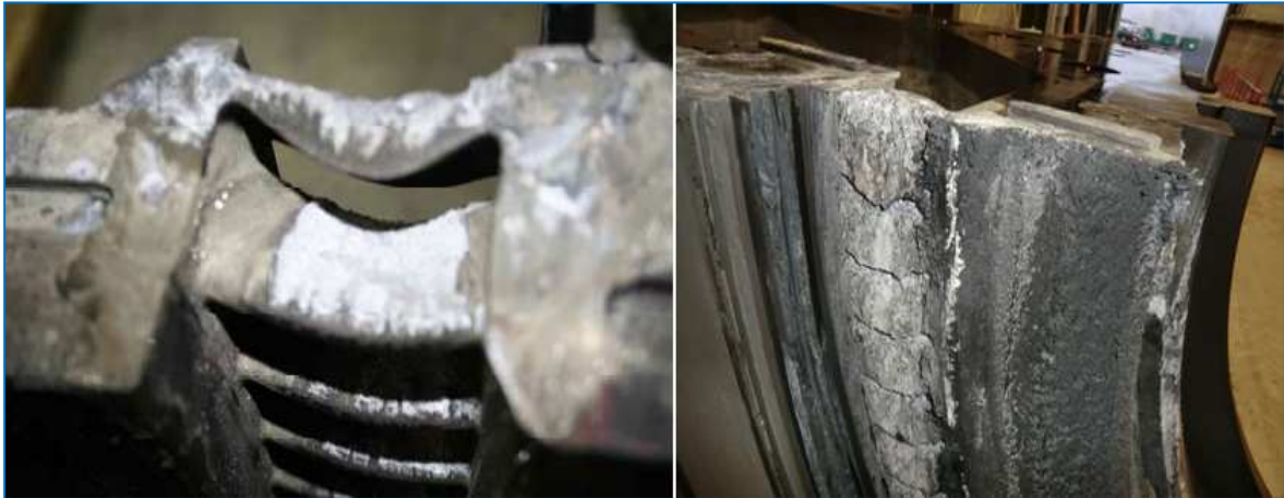
Figure 4.6 Left, scaling on the first stage stator blades in turbine 2 at Hellisheiði power plant. Right, scaling on the first stage stator blades in turbine 3 at Hellisheiði power plant [41].
