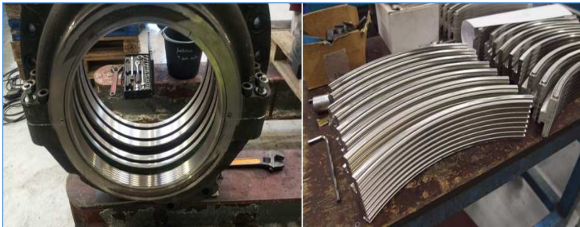
Figure 4.30 Left, repaired casing with labyrinth packing manufactured by Vélvík ready for installation. Right, new labyrinth seals for a labyrinth packing made by Vélvík ready for installation [41].
