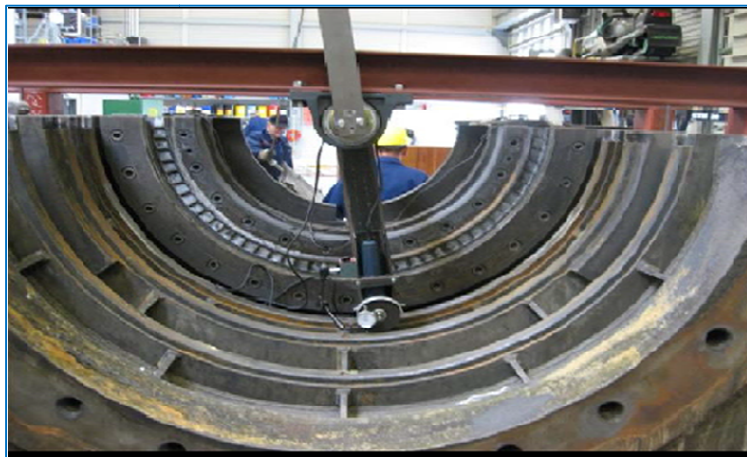
Figure 4.33 Polishing machine to polish diaphragm attachments in a casing of a steam turbine [41].
