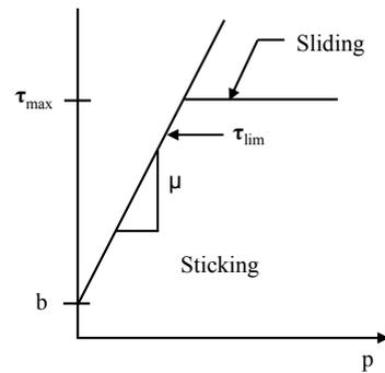
Figure 2: The Coulomb friction model in Ansys [1].
