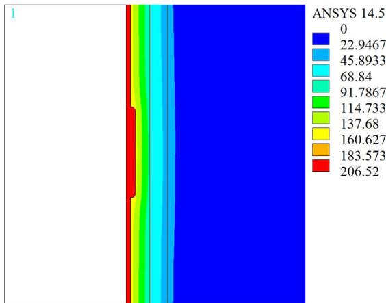
Figure 3: Temperature distribution 2.5 hours after discharge (°C).
