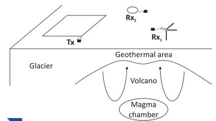
The loop will be placed about 15 km away from Grímsvötn and the transient magnetic field recorded on a dense net in the central area. In order to illuminate the sub-surface resistivity structure from different directions, at least two different source locations will be used.
