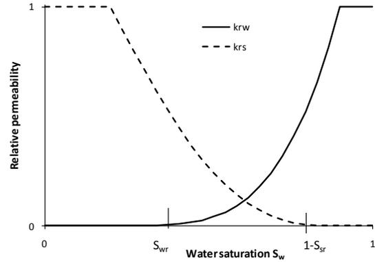
Figure 4: Relative permeability curves showing the "cut offs" of the residual saturations of the two phases
