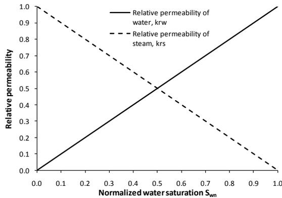
Figure 3: The theoretical X-curve, showing the relative permeabilites of water and steam as functions of the normalized water saturation
