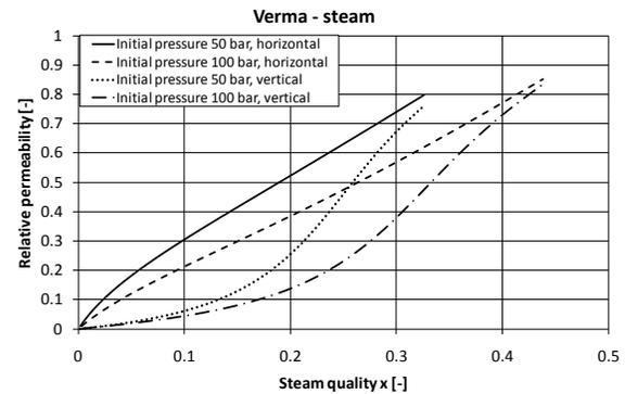
Figure 11: The relative permeabilities for steam as functions of steam quality when the Verma curves are used
