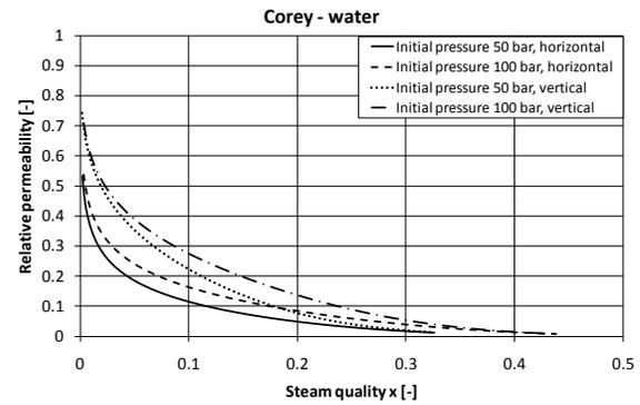
Figure 10: The relative permeabilities for water as functions of steam quality when the Corey curves are used
