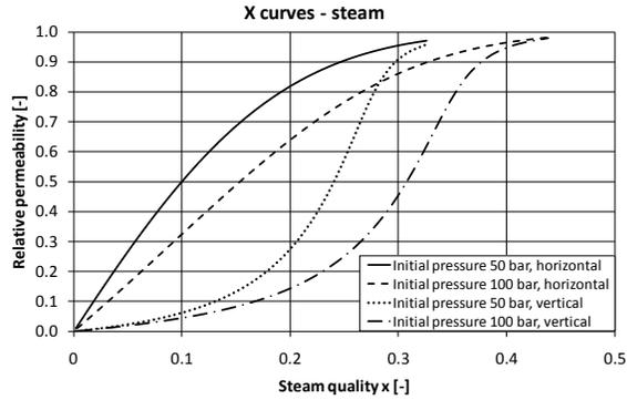
Figure 7: The relative permeabilities for steam as functions of steam quality when the X-curves are used
