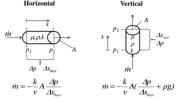
Figure 1: Representation of a one dimensional one phase flow of a fluid through a porous flow channel in different flow directions
