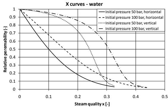
Figure 8: The relative permeabilities for water as functions of steam quality when the X-curves are used
