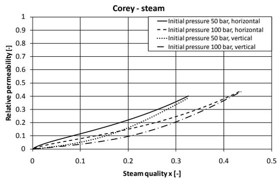
Figure 9: The relative permeabilities for steam as functions of steam quality when the Corey curves are used
