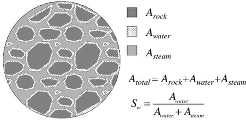
Figure 2: A cross section of a porous flow channel containing water and steam
