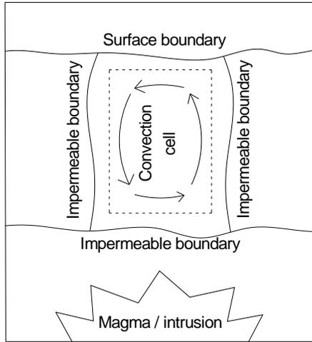
Figure 5: A convective geothermal reservoir where the reservoir fluid flows through the permeable reservoir. The fluid gains heat from the magma below and is cooled at the surface.
