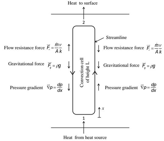
Figure 6: A convection cell and the corresponding forces acting on the fluid flowing in a streamline
