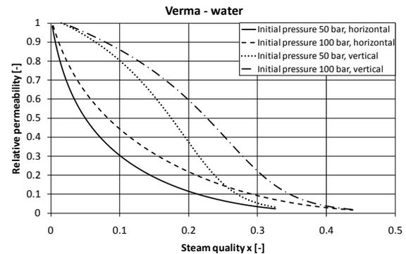
Figure 12: The relative permeabilities for water as functions of steam quality when the Verma curves are used
