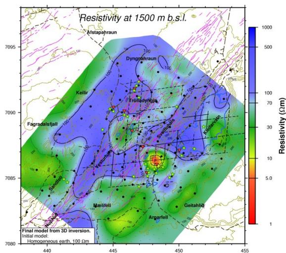
Figure 14: Resistivity at 1500 m b.s.l. Initial model explained in Figure 10 and legend in Figure 7.
