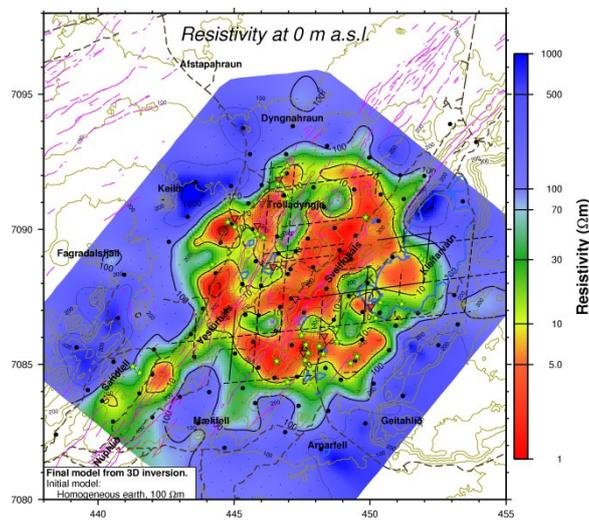
**Figure 10: Resistivity at sea level. Initial model: homogeneous earth of resistivity 100 Ωm. Legend is explained in Figure 7.**
