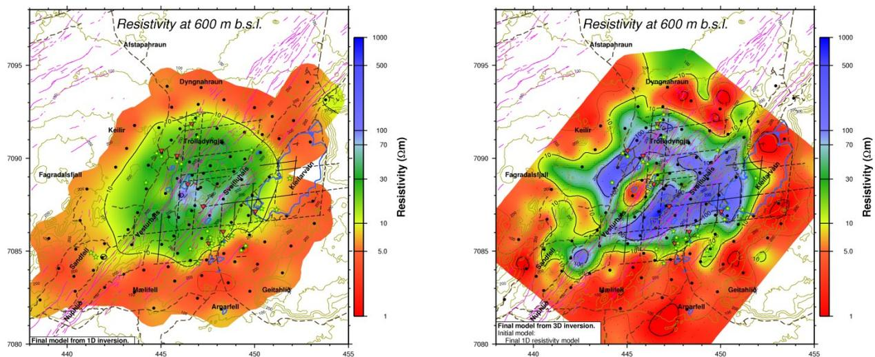
Figure 7: Resistivity models at 600 m b.s.l.: Based on 1D model (left panel) and 3D model using the 1D model as an initial model (right panel). Wells deeper than 300 m are denoted by red filled triangles, fumaroles by green/yellow stars and fractures and faults by magenta lines Solid and broken straight black lines show possible fracture zones, inferred from seismicity.
