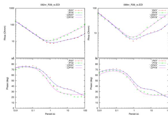
**Figure 4: An example of data fit: A comparison of the (re-sampled) processed data (dots) for two soundings presented as apparent resistivity and phase and the calculated response of the final model from the inversion (unbroken lines).**
