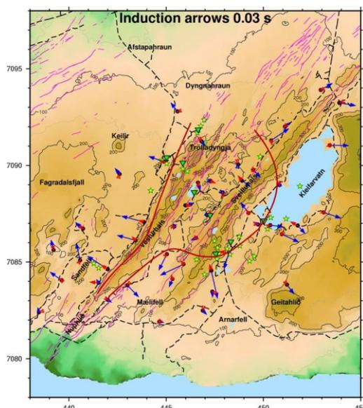
**Figure 20: Induction arrows for the period 0.03 s. Blue arrows denote the real part and red arrows the imaginary part. Thick dark red lines denote presumed boundaries of a good conductor according to the induction arrows. Legend is explained in Figure 19.**
