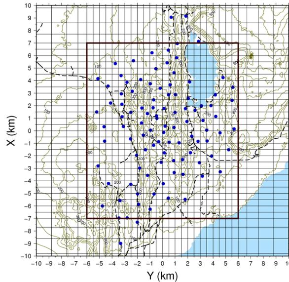
**Figure 3: The central part of the model grid mesh and the coastal line of the Reykjanes peninsula. Coordinates are km in the internal (local) coordinate system. The heavy black lines mark the area of 12 x 14 km and within it the thin lines mark a 500 m x 500 m grid. The 102 MT sounding locations are shown as blue dots.**
