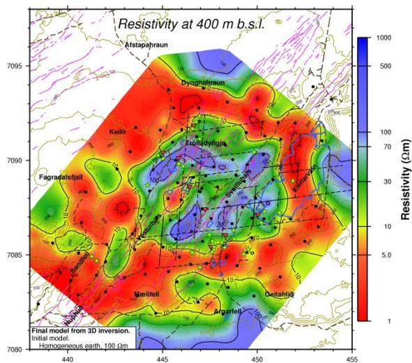
Figure 12: Resistivity at 400 m b.s.l. Initial model explained in Figure 10 and legend in Figure 7.
