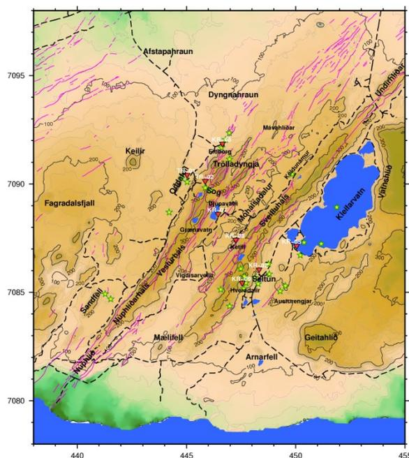
**Figure 2:** An overview of the survey area and the main landmarks. Wells deeper than 300 m are denoted by red filled triangles, fumaroles by green/yellow stars and fractures and faults by magenta lines. Blue color denotes the ocean and lakes.
