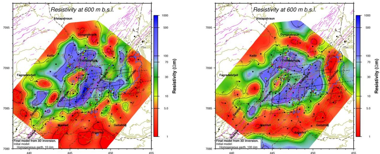
Figure 8: Resistivity models at 600 m b.s.l.: Based on 3D models, using homogeneous earth as an initial model with 10  $\Omega\text{m}$  (left panel) and 100  $\Omega\text{m}$  (right panel). Legend is explained in Figure 7.
