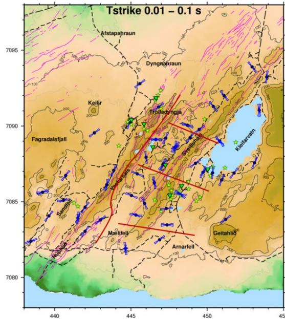
**Figure 19: Rose diagram of the Tipper strike for the period, 0.01–0.1 s. Thick dark red lines indicate zones of different dominant strike directions. Wells deeper than 300 m are denoted by green filled triangles, fumaroles by green/yellow stars and fractures and faults by magenta lines.**
