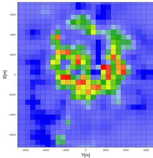
Figure 5: Raw model: resistivity at 100 m depth.
